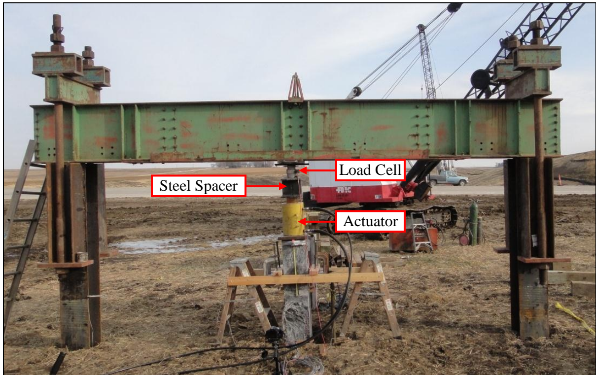
Figure 5-31: Completed Axial Load Test Set-up
