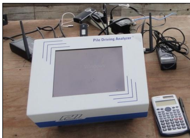
Figure 5-5: PDA Unit Provided by the Iowa DOT
