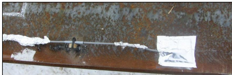
Figure D-2: Installed Weldable Strain Gage
