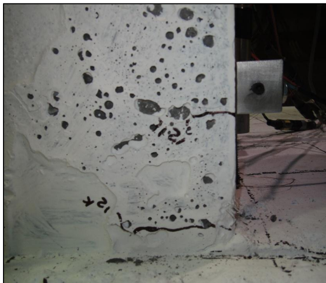
Figure 4-22: Hairline Tensile Cracks that Developed on the UHPC Pile in UPAC-2 at the 12 kip Lateral Load Step with a 100 kip Axial Load
