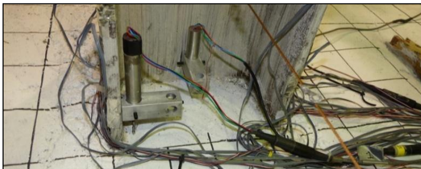
Figure 4-15: LVDTs used Near the Base of the Test Pile during Laboratory Testing
