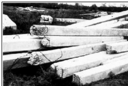
Figure 1-2: Concrete Piles Damaged by Difficult Driving Conditions (DiMillio 1998)
