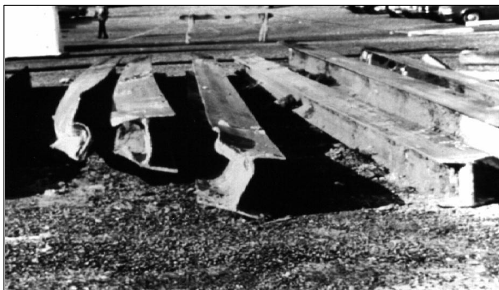
Figure 1-4: Damaged H-Pile Toe (Hannigan et al. 2006)
