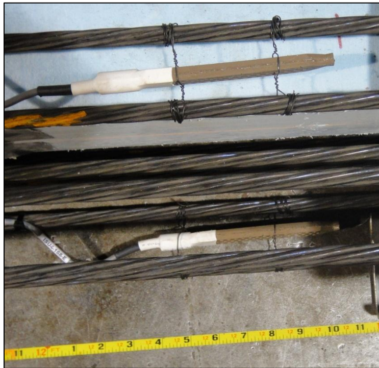
Figure 5-38: Suspended Embedded Strain Gages
