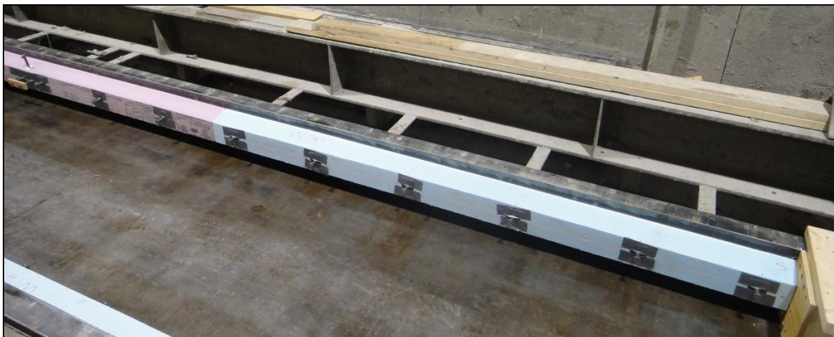
Figure 5-3: Locations of Steel Plates Embedded into P4
