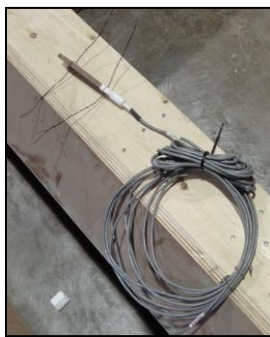
Figure 5-1: Embedded Concrete Strain Gage
