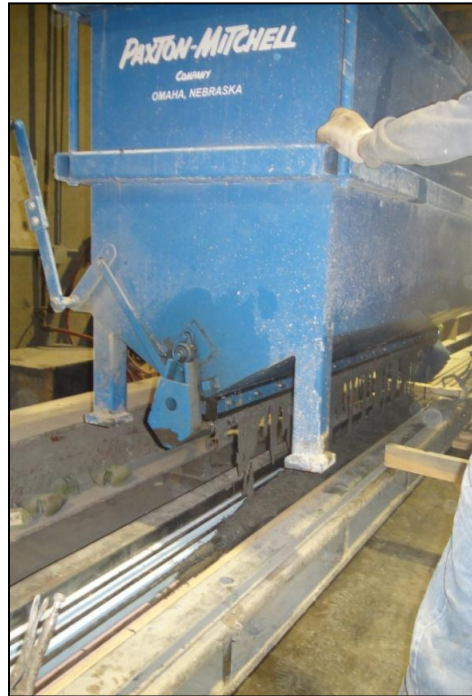
Figure 5-14: Pouring the UHPC from the Bin into the Forms
